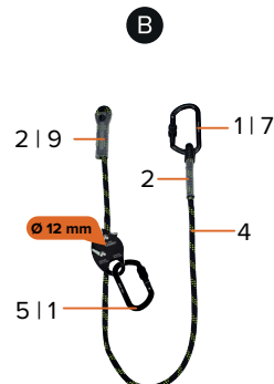
FS630 EN353-2:2002 MAX. LOAD 140 kg (compatible with FS33320/ KITS)
